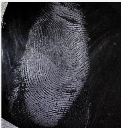
Fingerprint in blood on a glass developed, fingerprint by Mikrosil, Placed inside of the lightbox.
