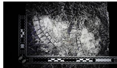
Photographing shoeprint in blood on aluminum foil, developed with Wet Powder White ; using one light source and Polarization filters
