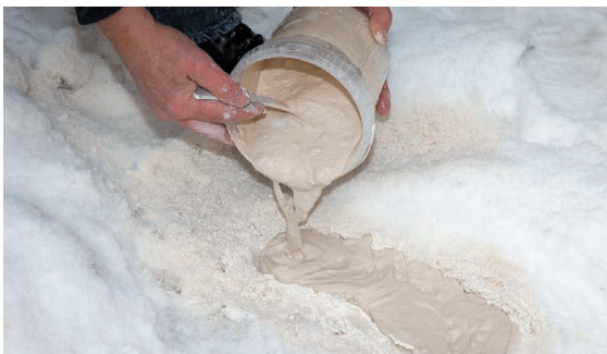
3. When the plaster starts to set, pour directly into the impression, working time approx. 30 sec. (at low temperature cover the poured plaster with newspaper).
