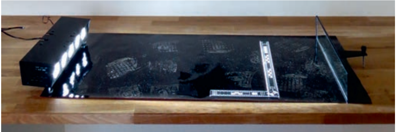
Photographing shoe prints in dust with low oblique light using the reflecting mirror. The mirror will give you more even light with better contrast.
