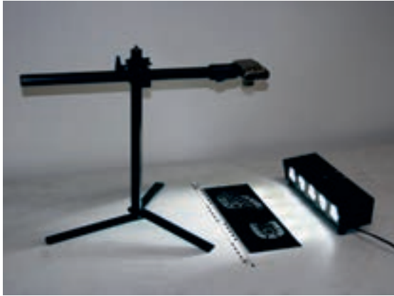
Using the light stand for photographing a gel lifting film with low oblique light
