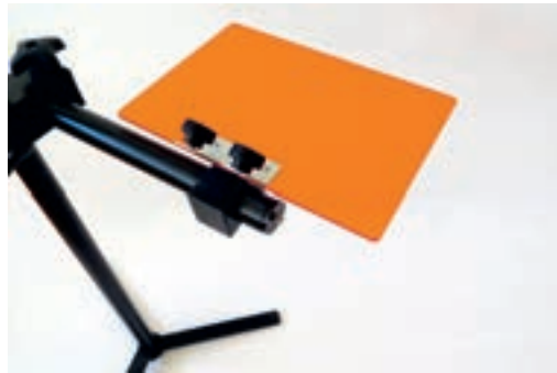
The orange viewing filter can also be attached on the stand using the small plastic clamp.
