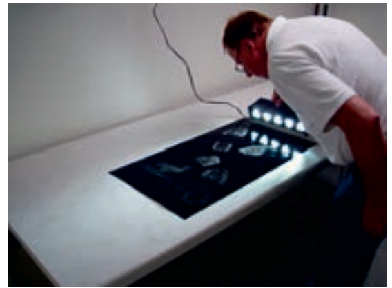
Examining an electrostatic film for shoe prints using the handheld Versa Light MAX
