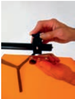
The orange viewing filter can also be attached on the stand using the small plastic clamp.
