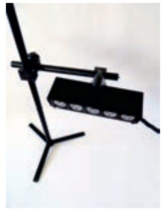
To mount the light source on the stand. Use the large plastic clamp and attach it to the handle which is mounted on the lamp, as illustrated.
