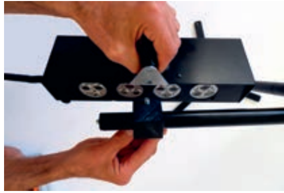
To mount the light source on the stand. Use the large plastic clamp and attach it to the handle which is mounted on the lamp, as illustrated.
