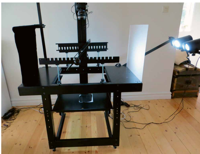
Photographing a shoeprint in blood on a wrinkled paper, secured with Black MIKROSIL and silicone paper using coaxial lighting. The acrylic plastic board and the two light sources with diffusion filters give an extreme soft light. That light is reflected from the Transparent mirror, which is mounted in approximately 45 degrees between the camera and the print. The Black velvet textile on the left side is blocking unwanted reflections and gives a black background in the photo.
