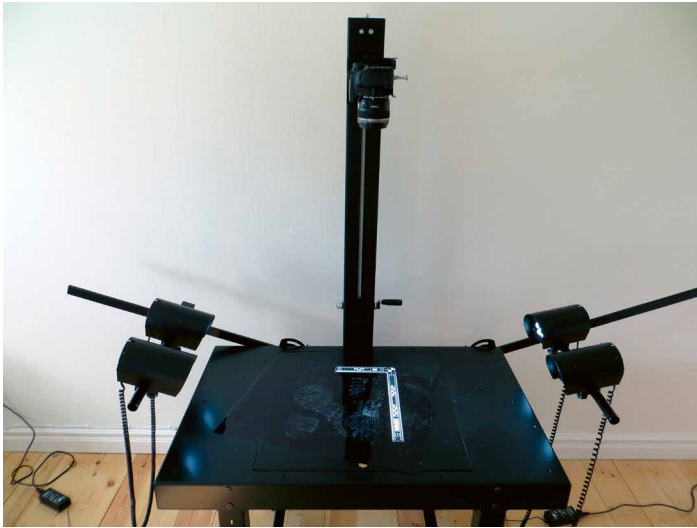
Photographing shoe print in dust with low oblique light.
