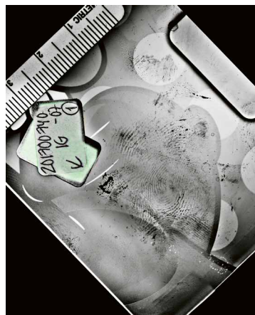
This is the result of an untreated fingerprint on a bathroom scale photographed with the coaxial light technique, the image on the left shows normal light exposure and the image to the right shows the same area with the coaxial lighting setup as shown above.
