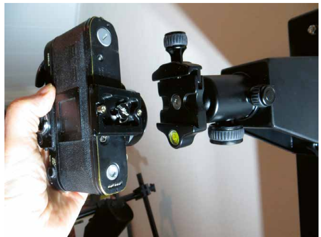
The release plate of the Ball Head is mounted on the camera, which easily locks on the Ball Head with the fixing screw.
