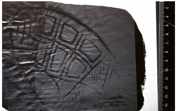
Photographing a shoeprint in blood on a wrinkled paper, secured with Black MIKROSIL and silicone paper using coaxial lighting. The acrylic plastic board and the two light sources with diffusion filters give an extreme soft light. That light is reflected from the Transparent mirror, which is mounted in approximately 45 degrees between the camera and the print. The Black velvet textile on the left side is blocking unwanted reflections and gives a black background in the photo.
