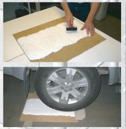
Making a three-dimensional test impression from a tire, with a wet tire you will get a better release.
